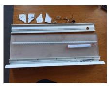
Step 5 Solder the cable off the PCB
