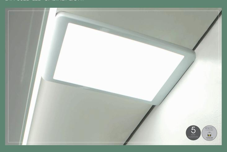
The slimline Sirius tablet style cabinet light offers a superior light output, and has no visible LED points due to the diffused style cover. The panel is only 6mm thick, and is easily installed by fixing the metal plate to the cabinet, and the light magnetically attaches itself to the plate. It can also be easily removed for cleaning. A 500mm connecting cable is available to link each light together.
