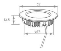
Cut out size if recessed 57mm Spacer Depth 16mm
