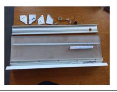
Step 3 Solder the cable off the PCB
