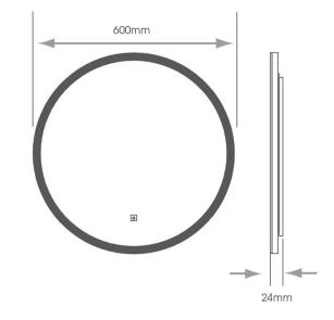
The Oslo features a natural white (4000K) LED diffused illuminated border to the face of the mirror, which provides a uniform light output with no dark spots.
