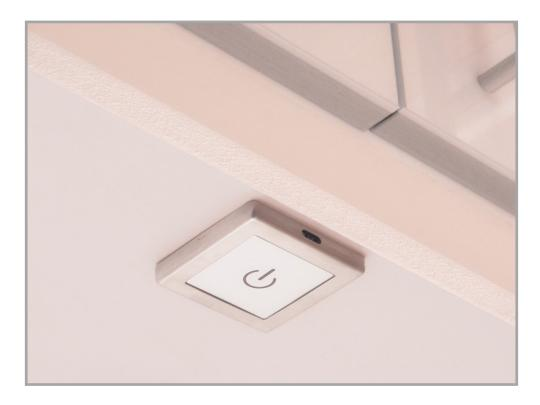
The touch dimmer is compatible with all of our 24Vdc lighting ranges. It offers a simple plug and play connection system, so lights can be controlled from a single switch. The unit incorporates a soft blue light to aid location in the dark and a surface mounted fixing method via 2 screws, which are hidden by the clip on a brushed nickel fascia plate.
