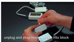
3. Unplug the receiver from the driver. The lights will go off. Plug the receiver back into the driver. The lights will come on again. When the lights come back in you have 3 seconds to complete step 4.
