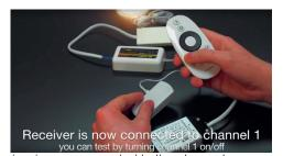
5. The receiver is now connected to the channel you synced it to. You can now test this by turning the channel on and off.
