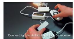
2. Connect the light to the distribution block on the receiver. Switch on the power to the driver and the light will come on.
