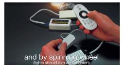
6. You can also test the remote by spinning the wheel, the lights should dim and brighten.
