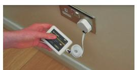
7. Plug the USB adapter into a socket (plug not included). Switch on and leave on. The lights should flash. The wifi device must now remain switched on, and within a radius of 30m from remote.
