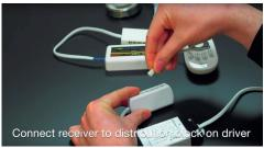
1. Connect receiver to the distributor block on driver
