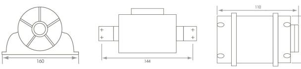
The shower fan kit in a highly reliable fan in a modular design for ease of installation and maintenance. The inline fan is designed to provide extraction levels that comply with the latest building regulations.
