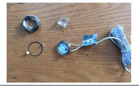
Step 2 Solder the cable off the PCB
