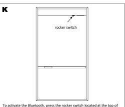
To activate the Bluetooth, press the rocker switch located at the top of the cabinet. The cabinet will give out a tone to confirm it is ready for pairing
