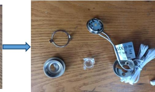
**Step 2** Solder the cable off the PCB
